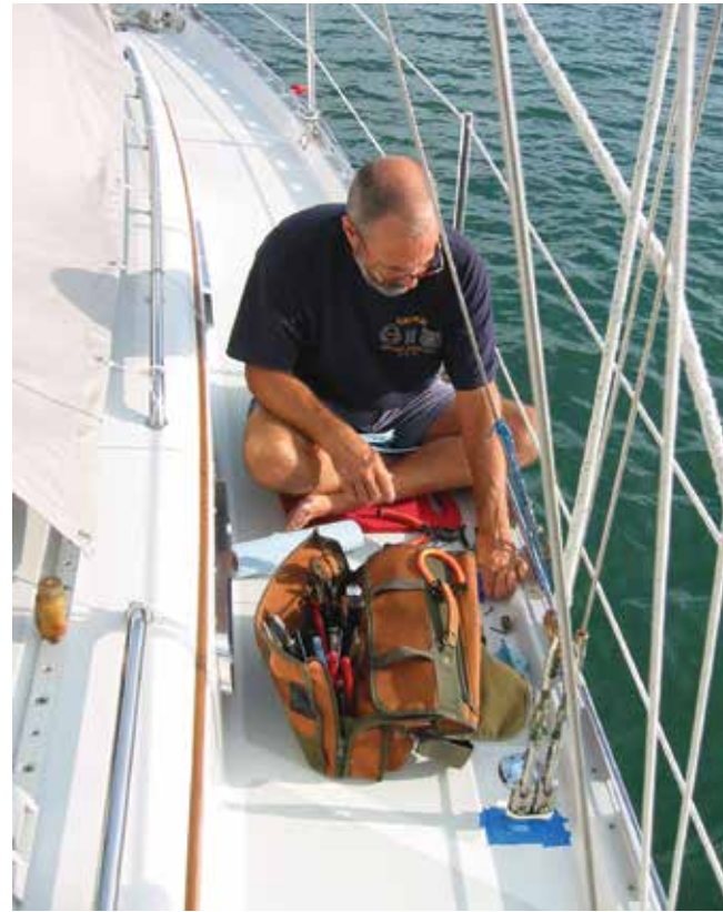
Repairs in exotic places—the author rebedding a chain plate.
